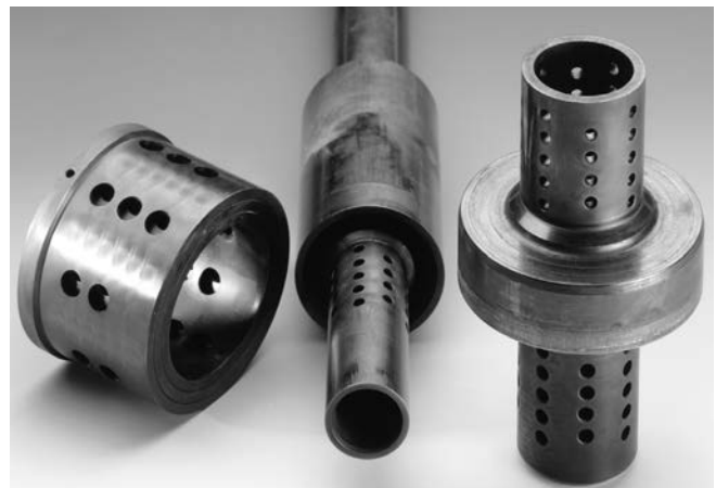
Internals of a leak-off valve ZK 213, DN 100, after 13 years of operation with p_1 = 374 bar (5420 psi), p_2 = 11 bar (159.5 psi), t = 172 °C (342 °F), \dot{m} = 35 kg/s (277800 lbs/h)
