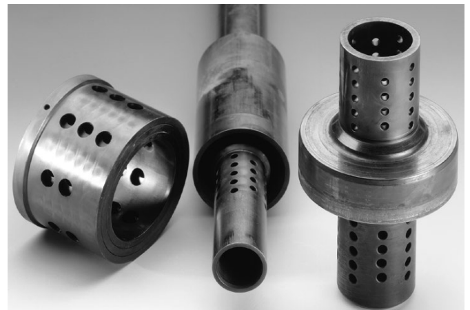
Internals of a leak-off valve ZK 213, DN 100, after 13 years of operation p_1 = 374 bar (5420 psi), p_2 = 11 bar (159.5 psi), t = 172^\circ\text{C} , \dot{m} = 35 kg/s
