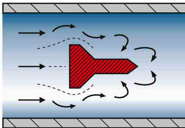
Vortex body with integrated baffle
