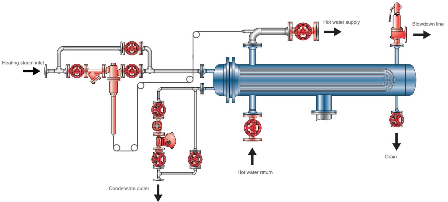
GESTRA offers various systems for controlling heat exchangers. Control on the steam side can be performed using self-acting temperature regulators (Clorius system), or controllers with electrical, pneumatic or electro-pneumatic actuation. For building heating systems, vertical heat exchangers with electrical controllers are frequently used on the condensate side.
