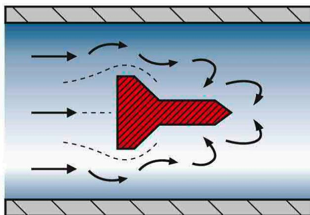
Vortex body with integrated baffle
