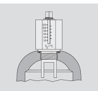
External adjusting device for BW 31, DN 15-40 mm (1/2-1)/2
