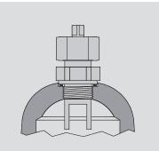
External adjusting device for BW 31a, DN 15-40 mm (1/2-11/2)
