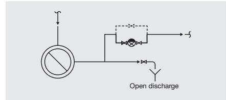
Installation in a bypass, open discharge
