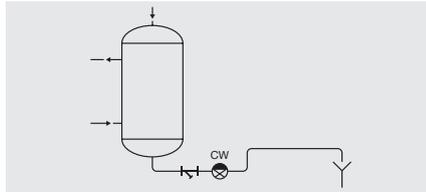
Application downstream of a counter-flow cooler
