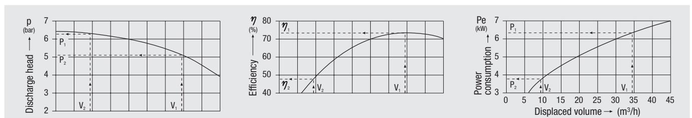
Savings in cooling water and pump energy by increasing the cooling-water discharge temperature.
