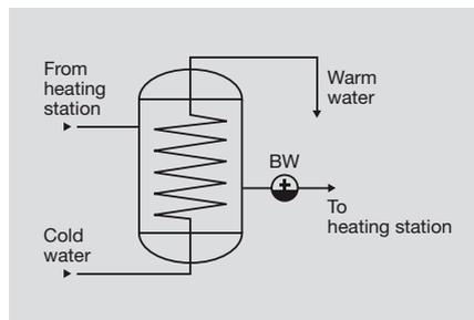
*Installation in the outlet line of water heater*
