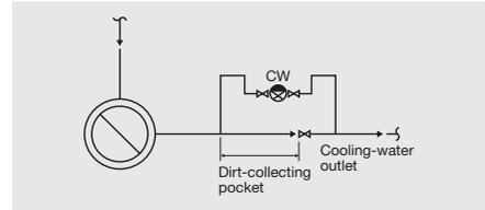
Installation in a bypass, closed system
