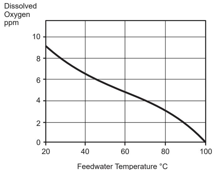
**Graph showing dissolved oxygen content of feed water at any temperature**
