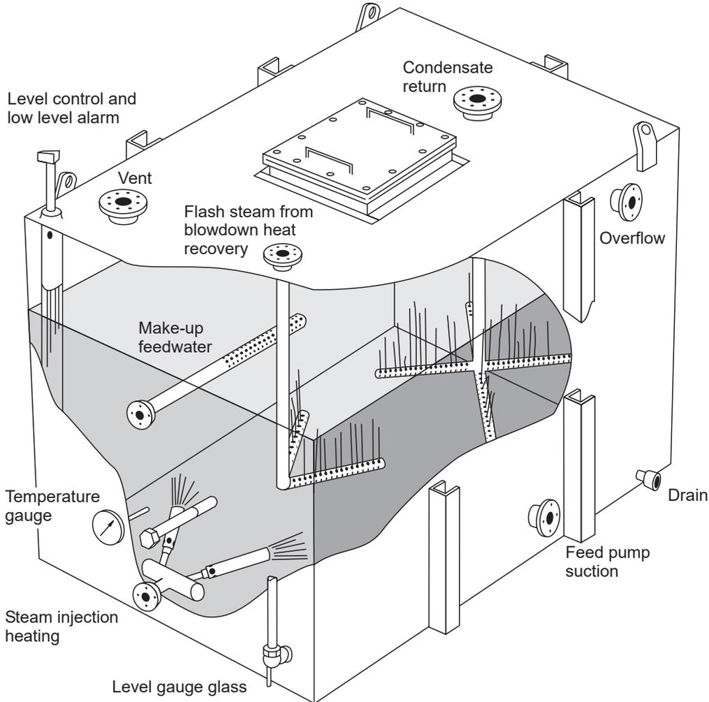
**The Semi-Deaerator conditions the boiler feedwater in a complete package unit which includes:**
