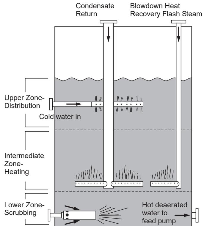
**Schematic layout of the Gestra Semi-Deaerator showing the three zones**
