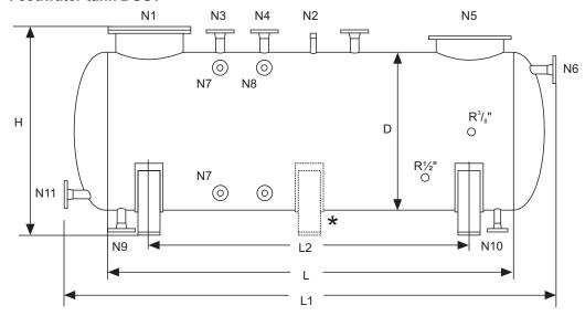
Typical Dimensional Details for Feedwater Tank DGST
