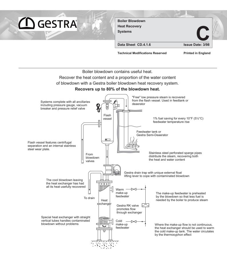
Ask us for a free survey to assess the potential for Boiler Blowdown Heat Recovery
