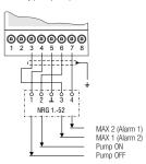
MAX alarm and pump (ON/OFF) / sensitivity (> 10 µS/cm) with NRG 16-36
