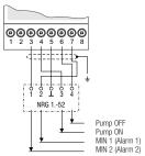
MIN/MAX alarm and pump (ON/OFF) / sensitivity (> 10  $\mu\text{S/cm})$  with 4 x NRG 16-4
