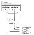
MIN1/MIN2 alarm and pump (ON/OFF) / sensitivity (> 10 µS/cm
