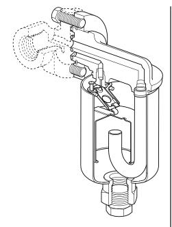
Sealed Inverted Bucket Steam Traps for use with Pipeline Connectors PC **UIB30**
