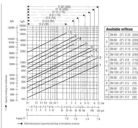
(Cold-water capacity  $\approx$  capacity of boiling hot condensate x factor F)
