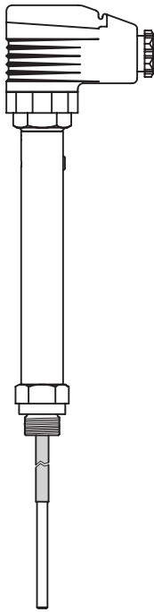
NRG 16-4 with four-pole connector
