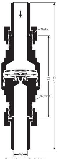
Design with union butt-weld nipples
