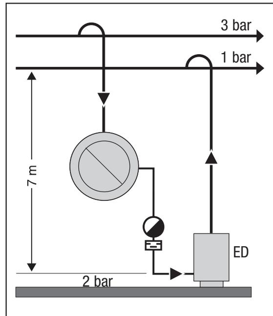
The condensate is pushed up to a higher level
