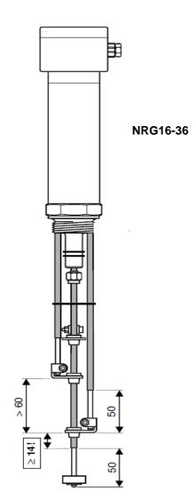
NOTE: The NRG16-36 is supplied as standard with metal surface extension clamps for use with water with Enclosure for Level Switches conductivities down to 0.5 microS/cm.
