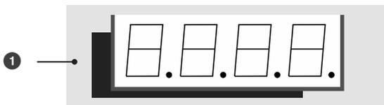
Fig. 23 1 Actual value display/error code/limit value, green, 4 digits
