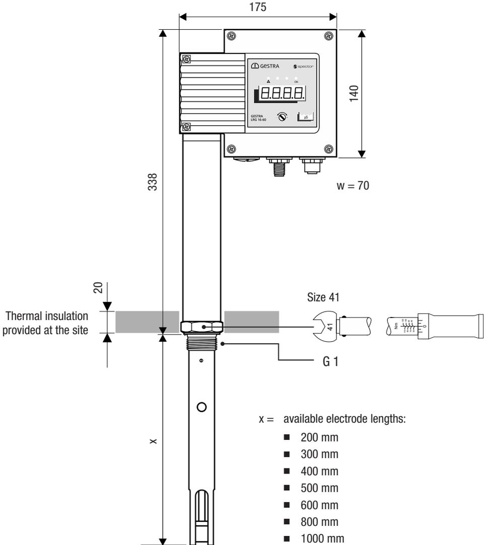
**Fig. 8** All lengths and diameters in mm
