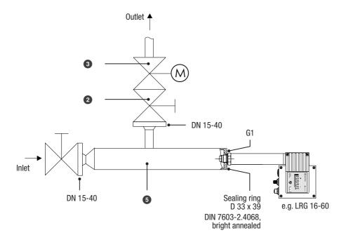
Fig. 16 All lengths and diameters in mm
