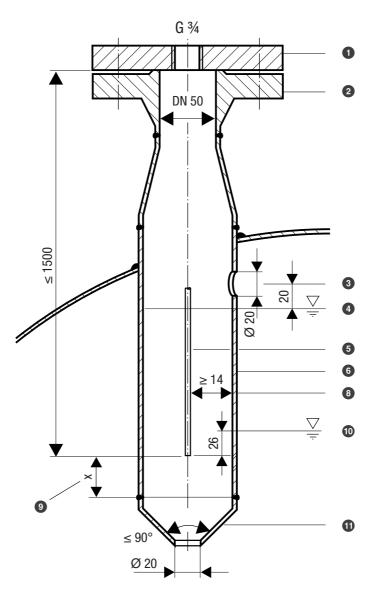
Protective tube (provided at the site) for internal installation, combined with other equipment from GESTRA AG.
