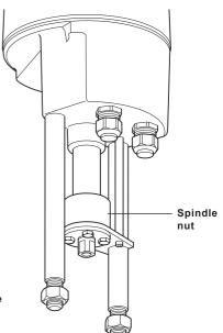
Fig. 33 Spindle nut maintenance
