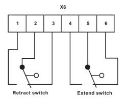
Fig. 25 AEL5951 auxiliary switches
