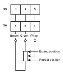
Fig. 24 AEL5953 2nd output from tandem potentiometer
