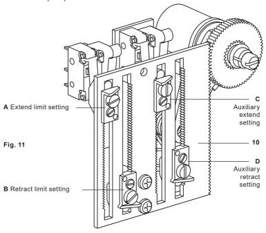
Section 3.6.6 shows how the switches are wired to the terminals. Fit the extend cam and the retract cam to position C and D respectively in Figure 11.
