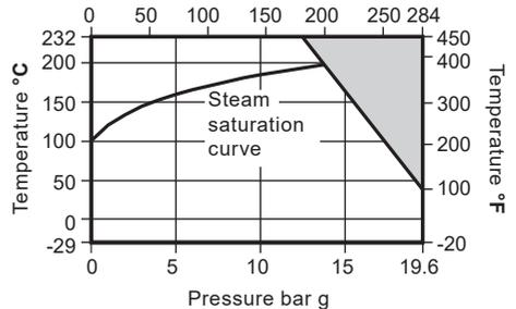
**Note:** When selecting a valve with a bellows sealed bonnet, the pressure/temperature limits of the bellows must be read in conjunction with the valve pressure/temperature limits shown above.
