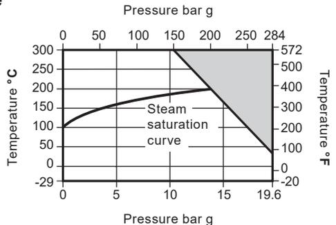
**Note:** When selecting a valve with a bellows sealed bonnet, the pressure/temperature limits of the bellows must be read in conjunction with the valve pressure/temperature limits shown above.
