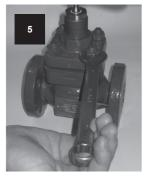
Using a spanner lightly and evenly tighten each bolt or nut by 45°, following the sequence illustrated in Figure 5, page 37.
