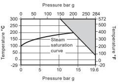
Note: When selecting a valve with a bellows sealed bonnet, the pressure/temperature limits of the bellows must be read in conjunction with the valve pressure/temperature limits shown above.
