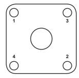
Fig. 5 Bonnet tightening sequence
