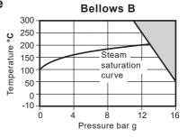
Note: When selecting a valve with a bellows sealed bonnet, the pressure/temperature limits of the bellows must be read in conjunction with the valve pressure/temperature limits shown above.
