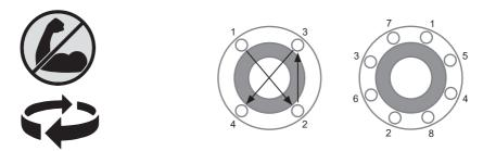
Do not over tighten. Use correct torque figures.
