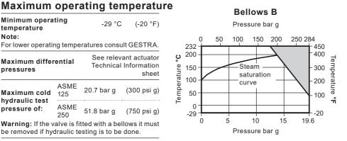
Note: When selecting a valve with a bellows sealed bonnet, the pressure/temperature limits of the bellows must be read in conjunction with the valve pressure/temperature limits shown above.
