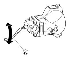
You can check the correct functioning of the equipment during operation using the GESTRA ultrasonic measuring unit VAPOPHONE<sup>®</sup> or TRAPTEST<sup>®</sup> (VKP 40 and VKP 40plus).
