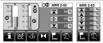
For each setpoint press the green button. Use the on-screen numberpad Screen display 2 to enter the desired percentage value.
