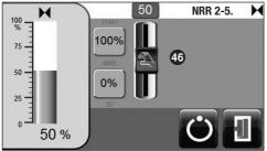
Screen display 7 Switch back to automatic operating mode and scroll back.
