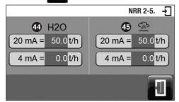
For each flowrate setting press the green button. Use the on-screen numberpad to enter the desired value
