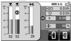
To enter the evaluation factor press the green button. Use the on-screen numberpad to enter the desired value.
