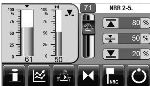
Use the hand slider to change the position of the control valve. The green button indicates the valve opening in %. Or press the green button and enter the desired valve opening in % in the numberpad.
