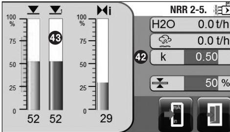
To enter the evaluation factor press the green button. Use the on-screen numberpad to enter the desired value. The factor evaluates the influence of the difference (steam flowrate - feedwater flowrate) on the measured level signal.
