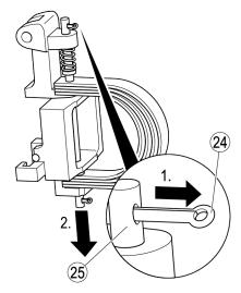
➤ Push the retaining rod (25) through the holes in the new slider (14), in the thermostat bracket (5) and through the washer (26), as shown.
