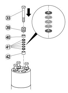
To mount the stuffing box packing do not tighten the bolts any more.
