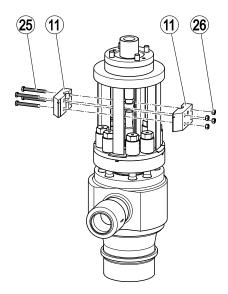
You can now remove the mechanical connection for the actuator.
