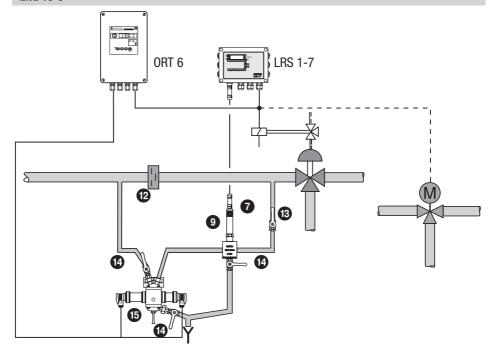
Conductivity electrode LRG 16-9 with measuring chamber for installation in a bypass together with the measuring sensor ORG 12 / 22 of the oil & turbidity detector OR 52-5 / OR 52-6.
