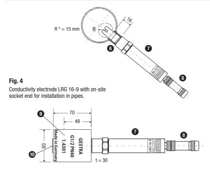
**Fig. 5**Conductivity electrode LRG 16-9 with measuring chamber for installation in pipes.
