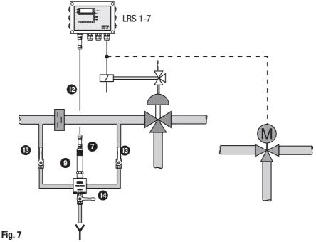
Conductivity electrode LRG 16-9 with measuring chamber for installation in a bypass
