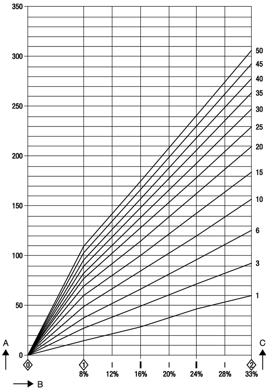
Flow diagram for DN 15 to DN 32, capacity range up to 1,020 kg/h
