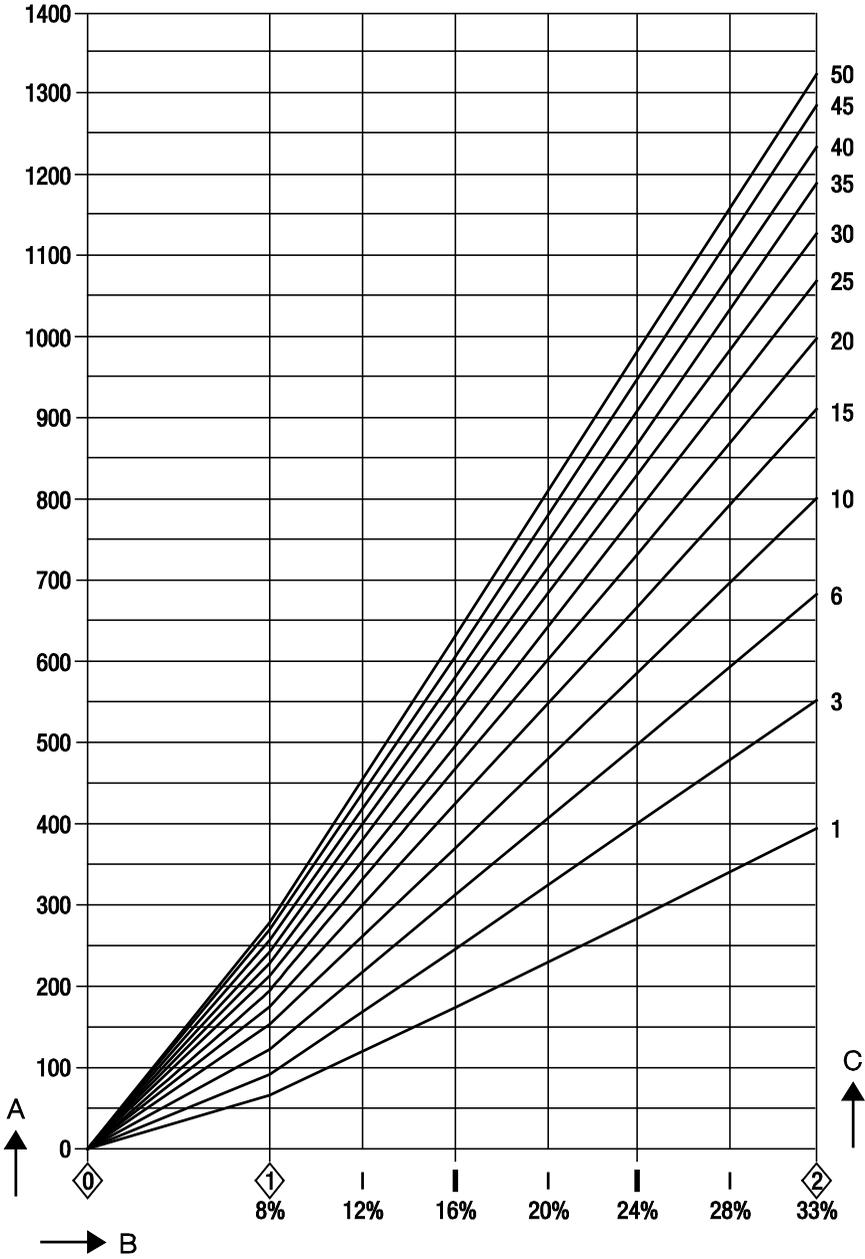
Flow diagram for DN 40 and DN 50, capacity range up to 4,500 kg/h
