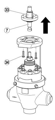
Unscrew the spindle out of the bearing if necessary.
