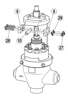
You can now remove the mechanical connection for the actuator.
