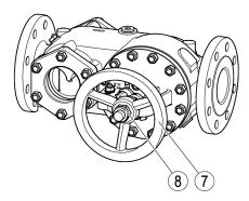
➤ To increase the flow, turn the handwheel anticlockwise.
