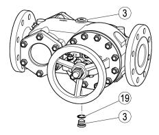
Coat the thread and contact surfaces with temperature-resistant lubricant. The lubricant must have the same properties as OKS 217.
