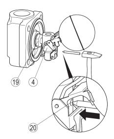
Attach the control unit to the body as described from page 16 onwards.
