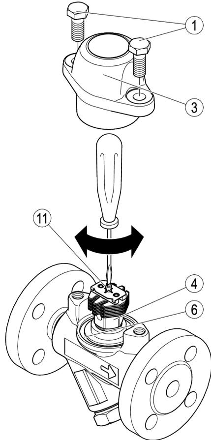
Different equipment types require different torques for tightening the screws.
